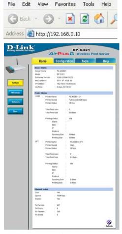
At the **Configuration** window, write down the **Port Names** for future reference. You will need this information later in the configuration process. The **Port Name** shown here is only an example.
